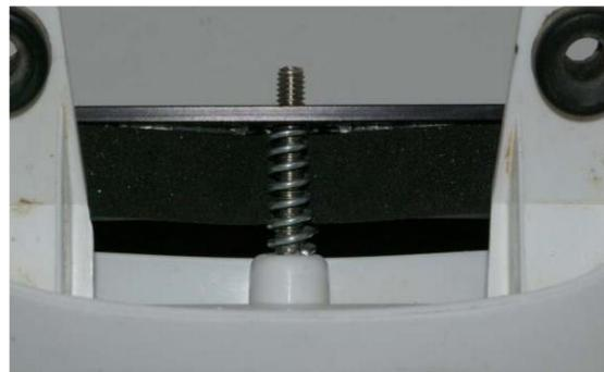
2. Assemble the silver bracket to the squadron bezel plate as shown in the exploded view below. Use the provided M5 button head bolt with the spacer and nut.
